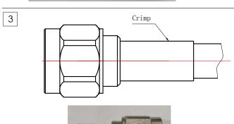
Insert the crimping tube into the shell and use a clamping tool to clamp the square (recommended clamping size 10.5)
