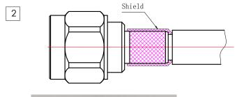
Push the above components into the main body, trim the shielding layer, and push up the crimping tube
