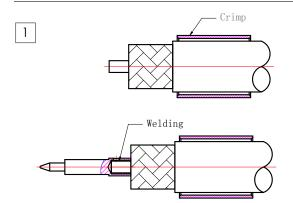
Peel off the cable as shown in the picture
