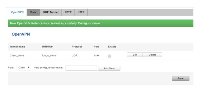
To see at specific configuration settings press "edit" button located in newly created configuration entry. A new page with detailed configuration appears, as shown in the picture below (TLS client example).
