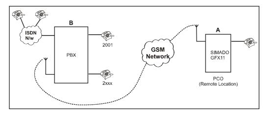
SIMADO GFX11 at the PCO is so configured that whenever a customer makes a call, the call is first made to the GSM Port of the PBX. Using DISA<sup>3</sup> services of the PBX, the final destination number dialed by the customer is dialed, and the call is made to the final destination. However, the customer needs to dial only the destination number.
