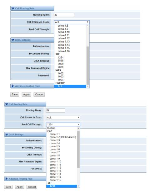
Figure 5-2 Example of Set up Routing Rule
