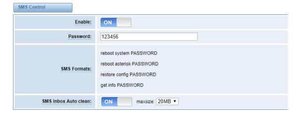
For example, SMS control password is 123456 which has nothing to do with the login password, you can send "get info 123456" to the CDMA module's phone number to get your gateway's IP information.
