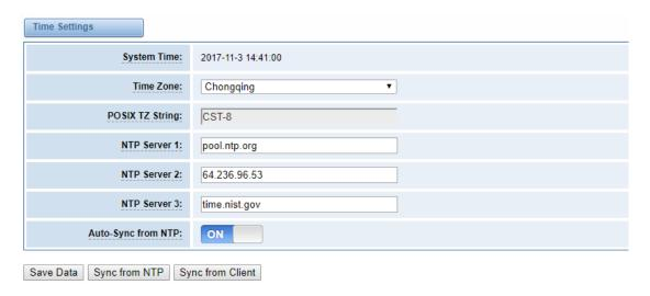
You can set your gateway time Sync from NTP or Sync from Client by pressing different buttons.
