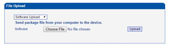
On the **Tools > Firmware Upload**, you can upload a firmware to upgrade the device. But you need to restart the device for the change to take effect.
