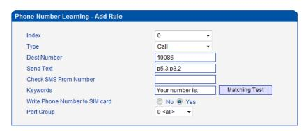
For make sure the configuration work, we can use the Matching Test. Input the "Your number is: 8618344144906" at Test SMS Text, press the Test, you will get the match result.
