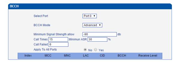
Note: When the actual number of failed calls reaches the set number, frequencies will be switched or when the actual answer-seizure ratio is less than the minimum answer-seizure ratio, frequencies will be switched.
