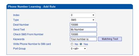
For make sure the configuration work, we can use the Matching Test. Input the "Your number is: 8618344144906" at Test SMS Text, press the Test, you will get the match result.
