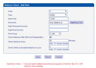
For make sure the configuration work, we can use the Matching Test. Input the "Your balance is 73.40\$" at Test SMS Text, press the Test, you will get the match result.
