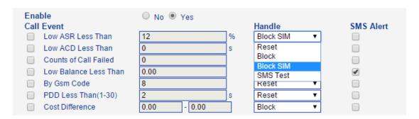
**Low ASR Less Than**: This value is the threshold of the ASR, once the exact ASR is lower than this value, the UC2000 port will be considered to be low ASR.
