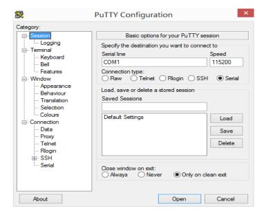
After finishing the above configurations, click the **Open** button to enter the maintenance interface of the console port. The username and password are the same with those of the web interface of device.
