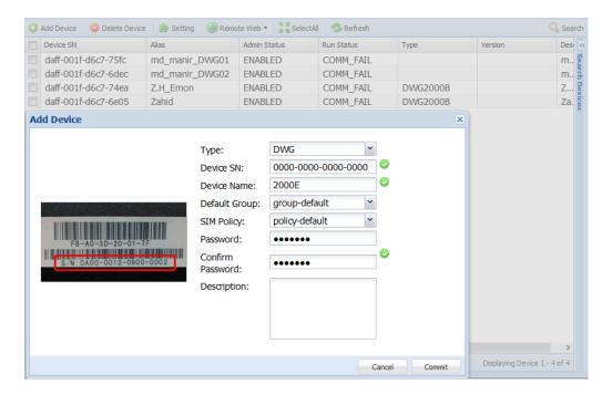
Device S/N is the device ID on gateway, find it on the page **system information**, as below:
