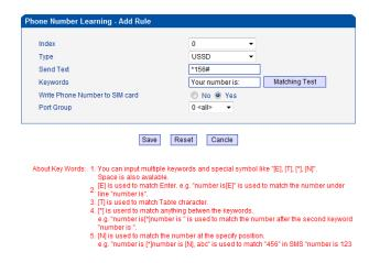
For make sure the configuration work, we can use the Matching Test. Input the "Your number is: 8618344144906" at Test SMS Text, press the Test, you will get the match result.
