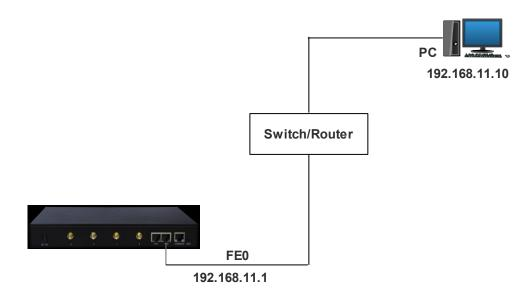
Note: UC2000-VE/F/G has two Ethernet ports (namely FE0 and FE1). The device can work normally when either of the ports is connected to PC. The IP address of device must be at the same network segment with that of PC.
