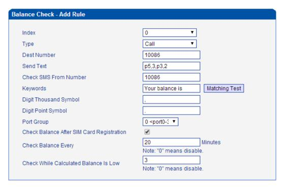
For make sure the configuration work, we can use the Matching Test. Input the "Your balance is 73.40\$" at Test SMS Text, press the Test, you will get the match result.
