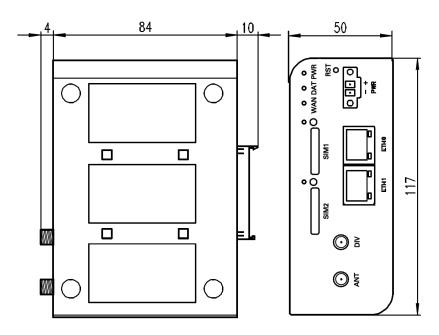
Figure 7: Basic dimensions of plastic box (bottom and front view)
