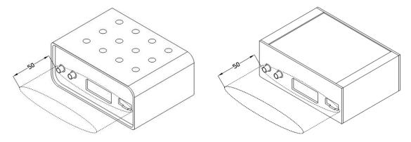
Figure 13: Space in front of connectors (plastic) Figure 14: Space in front of connectors (metal)
