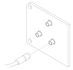
Figure 20: Connecting of the antenna
