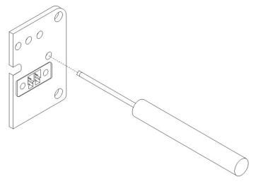
Figure 24: Router reset
