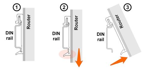
Figure 16: Removal from the DIN rail
