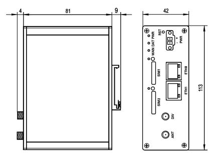
Figure 8: Basic dimensions of metal box (bottom and front view)
