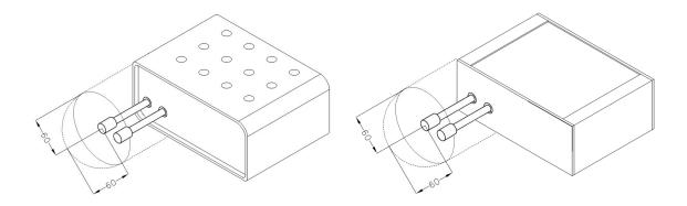
Figure 9: Space around antennas (plastic) Figure 10: Space around antennas (metal)
