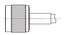
Push above patrs to the body in place. Trim shielding braids and cover it to crimp sleeve.
