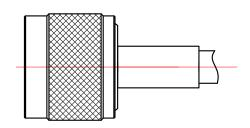
Crimp the crimp sleeve with crimp tool. Crimp tool with 5.6mm hex dies.
