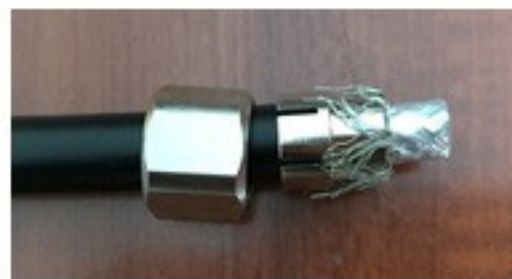
3. 将编织线向后弯折，漏出电缆锡箔层 Bend the braided wire backwards to leak the tin foil layer of the cable
