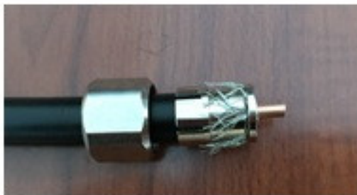
5. 紧贴内芯端面切电缆除锡箔层和绝缘层，漏出内导体 Cut the cable close to the end face of the inner core, except for the tin foil layer and insulation layer, and the inner conductor leaks
