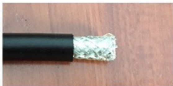
1. 环切外护套 15mm 左右； Circumcising outer sheath about 15mm
