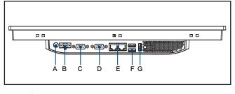
A. Power Switch B. DC-In C. RS-232
