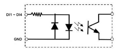
DI: isolated digital signal input channel GND: digital signal input
