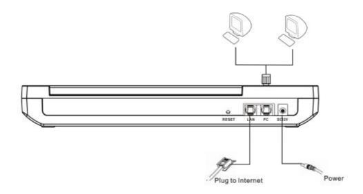
Connect the network cable linking the network to the LAN port, and the configuration PC or other shared PC in the network to the PC port. The LAN port can be connected to the ADSL Modem, Switch or Ethernet private lines. The SMB32 supports fixed IP and IP acquisition through DHCP and PPPoE.
