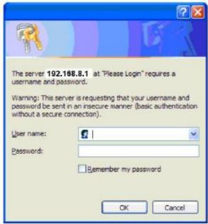
Enter the user name and password to log on the configuration interface (the initial user name and password are both "admin").
